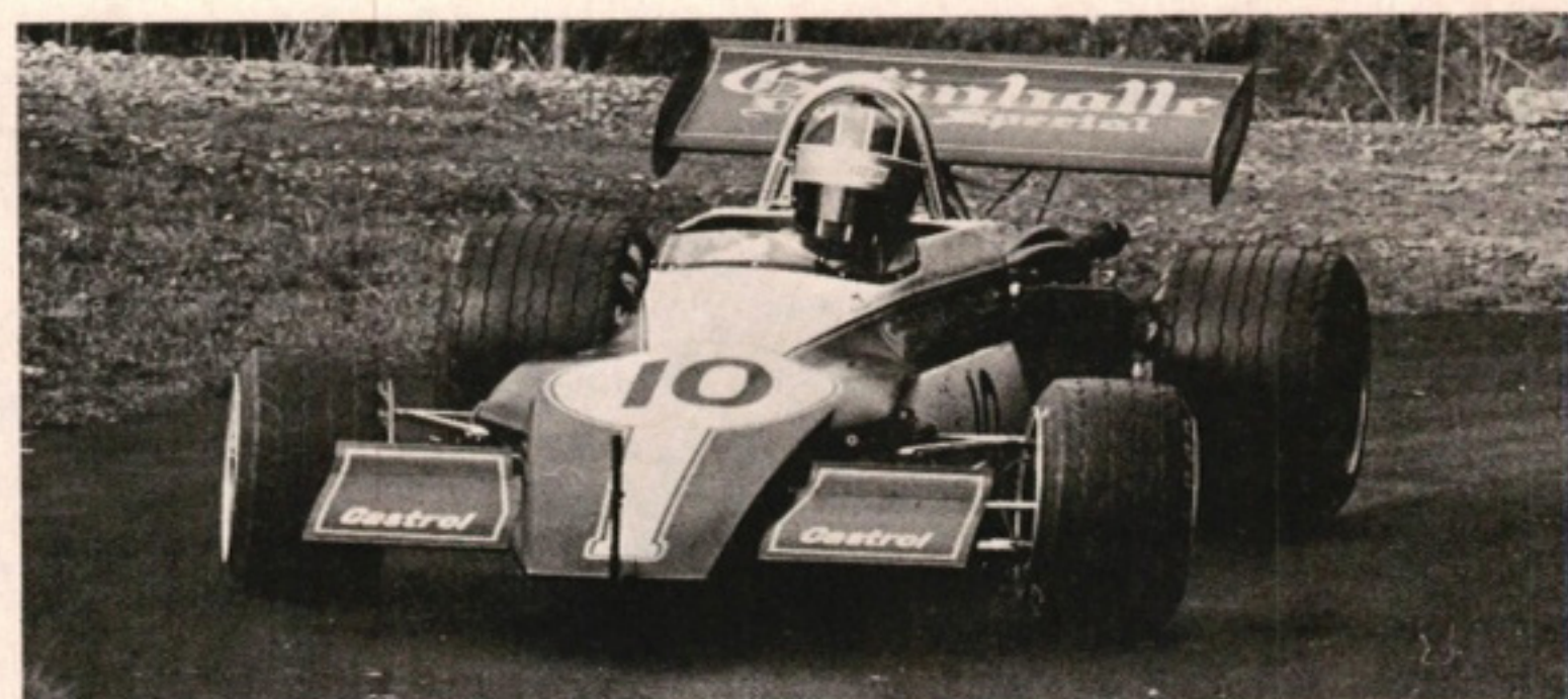
Chris Cramer has fitted the ex-Nick Williamson Hart BDA and Hewland box in an ex-works March 723 chassis with sponsorship from Grünhülle Lager (above). Mike MacDowel has bigger injection trumpets and rear wing on his 5-litre Brabham-Repco BT36X (below).
