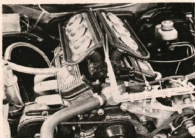
Ford's 320 bhp V6 engine.
