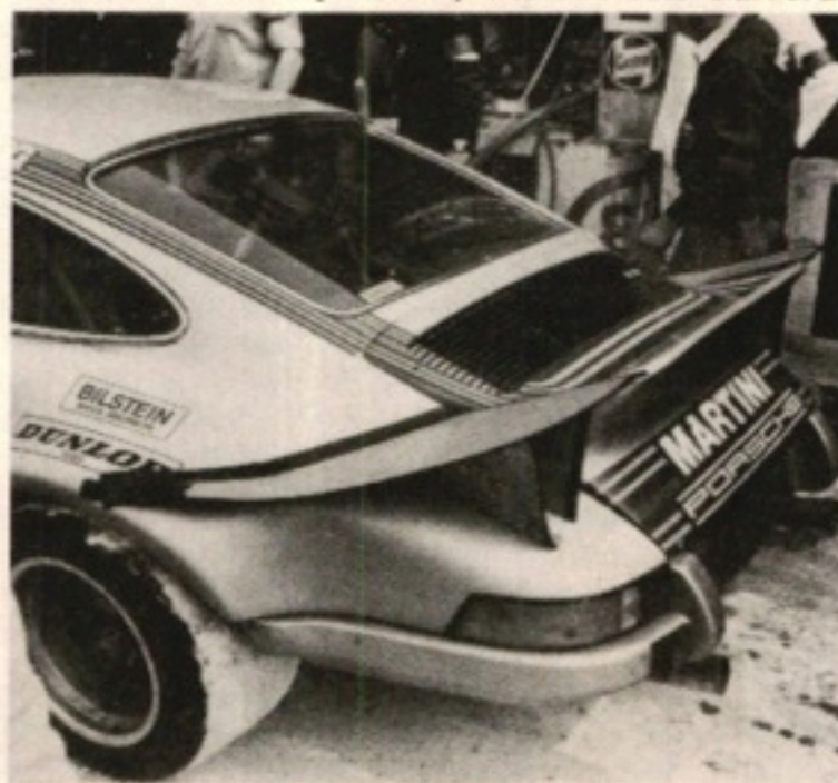
Additional rear spoiler of the Martini Carrera.
