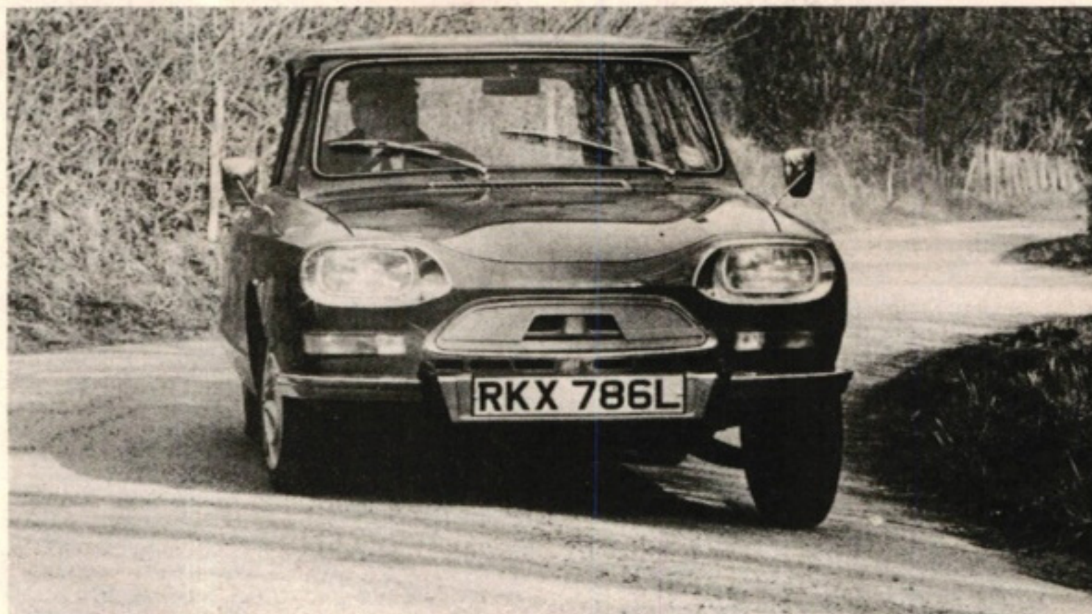
The car corners well, the angle of roll not being excessive due to twin anti-roll bars.
