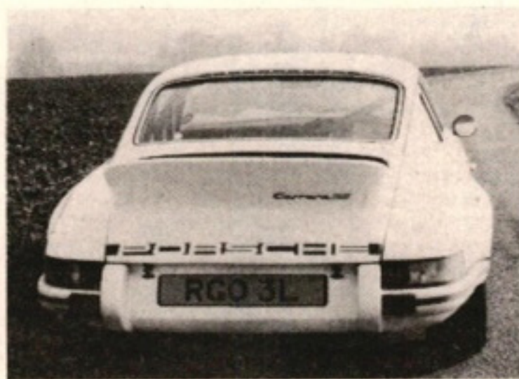
The Carrera's engine cover is in glass-fibre, above left. Right, cornering can be untidy, but the tail goes out well under power and is smooth and predictable. Below, the front spoiler was developed from the 908/3 sports/racer, the rear, quips the writer, from a Mallard!
