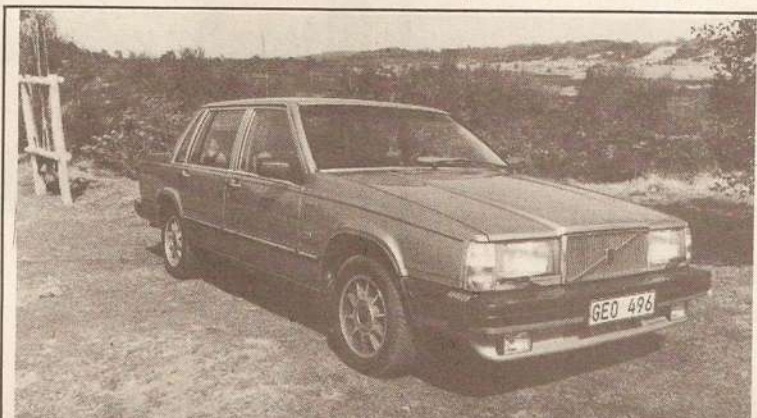
Though rather Detroit-like in its external styling, the new 760GLE Volvo — available at first only in 2.8-litre V6 petrol form — is a vast improvement over previous Volvos. Handling, ride and comfort are all excellent, and the interior sets new standards of efficiency and convenience. A 2.4-litre turbo diesel comes later this year, with a performance-orientated 173bhp turbocharged and intercooled petrol version to follow in the spring. Price of the well-equipped V6 petrol model is a keen £12,600.
