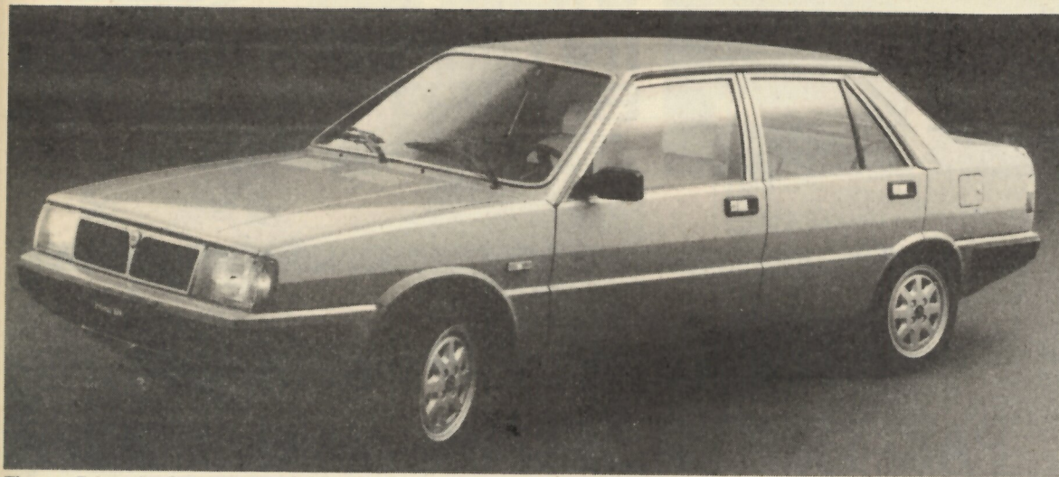
The new Prisma is of a conventional three-box design, although Lancia have opted for front wheel drive.
