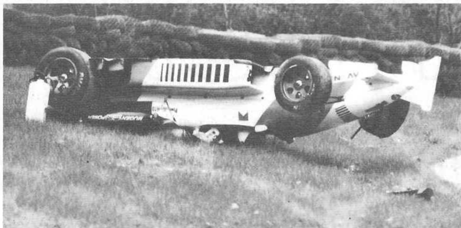
Allan McNish had a very lucky escape in practice at Brands Hatch, the Ralt RT33's roll hoop being pulled out of position as the car slid through the gravel trap.
