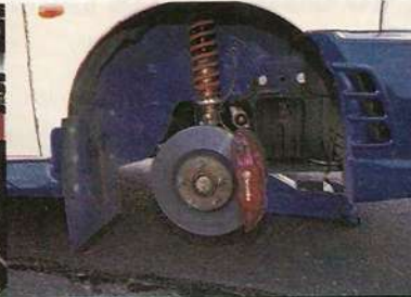
Standard suspension and stoppers are dumped for pukka rally items
