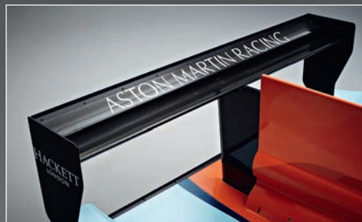
Rear aerodynamic treatment includes mandatory shark-fin for stability
