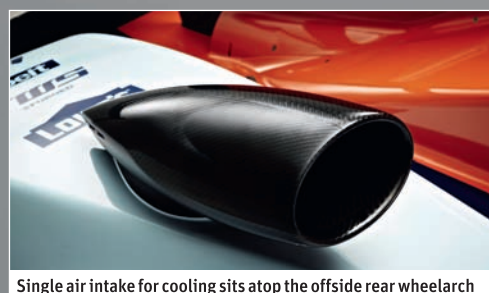
Single air intake for cooling sits atop the offside rear wheelarch
