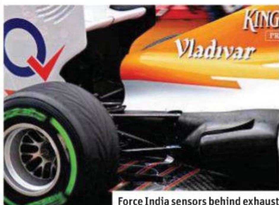
Force India sensors behind exhaust
