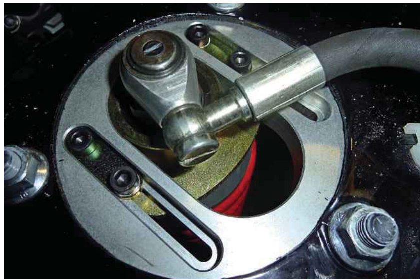
Left: top mounts are adjustable. Above and below: dampers carry three settings
