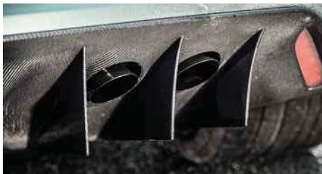
Above: exhaust pipes exit through carbon diffuser. Below: Bovington acclimatises to the One-77
