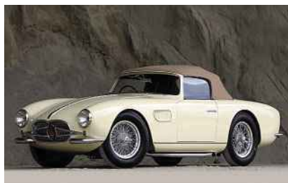
Above: one-off Maserati 150GT Spider features lightweight aluminium bodywork by Fantuzzi
