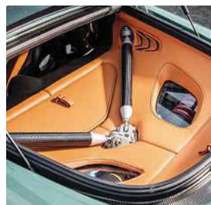
Above: inside of the front-hinged bonnet is covered with quilted silver sound-deadening material. Below left: just the two pedals. Below right: boot space impinged by chassis supports. Bottom: rear wing rises at 68mph, when the ride height also lowers by 15mm – changes that are reversed when the car drops below 31mph again
