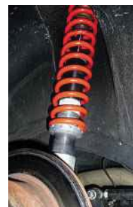
Left: top mounts are adjustable. Above and below: dampers carry three settings
