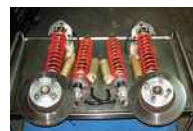
Left: top mounts are adjustable. Above and below: dampers carry three settings
