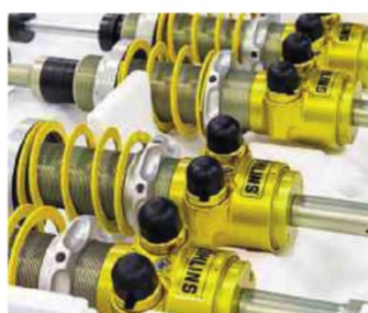
Right: bare shell with roll-cage installed. Above and below: Brembo braking system and Öhlins dampers will be fitted
