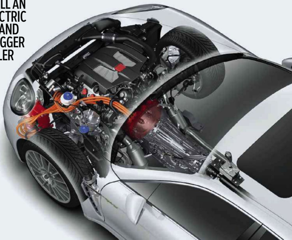
Left: 918's green tech brings weight penalty. Right: E-Hybrid runs 328bhp 3-litre V6 and 90bhp electric motor
