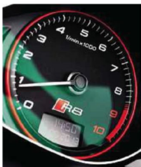
Above: R8's V10 hits its 518bhp peak at 8000rpm. Right: big engine contributes to the Audi giving away around 200kg to the V8-powered 458 and 12C. Far right: interior is relatively basic and is starting to feel a little outdated in this company
