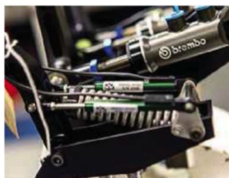
Right: bare shell with roll-cage installed. Above and below: Brembo braking system and Öhlins dampers will be fitted
