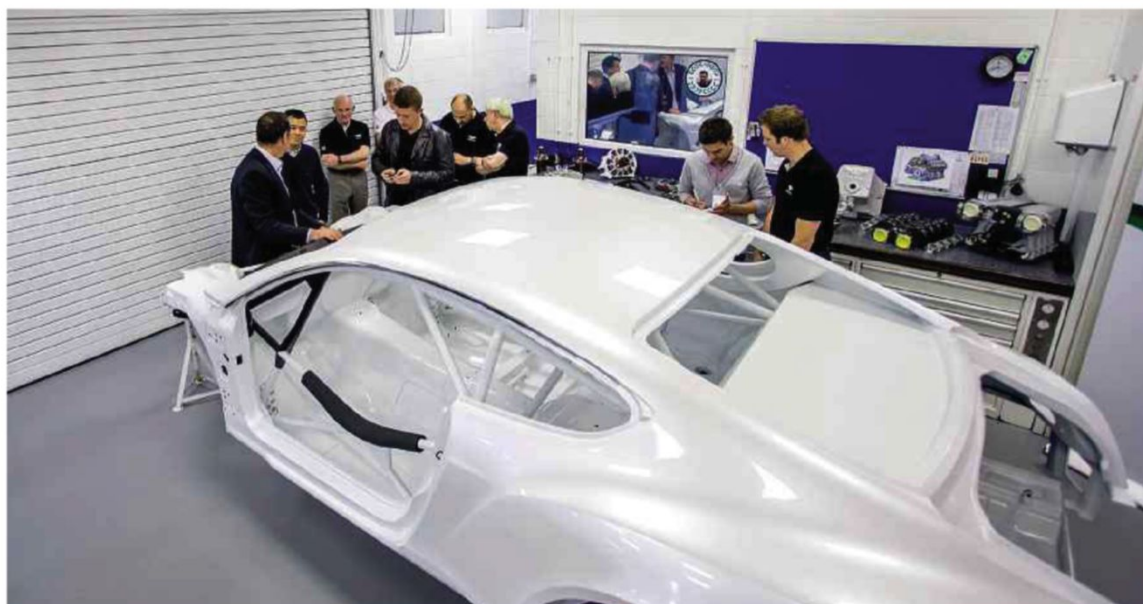
Right: bare shell with roll-cage installed. Above and below: Brembo braking system and Öhlins dampers will be fitted
