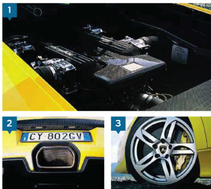
1: V12 is generally reliable – if you look after it. 2: LP640 swapped the twin tailpipes of earlier cars for a single huge exit. 3: Gallardo calipers of later cars improved braking
