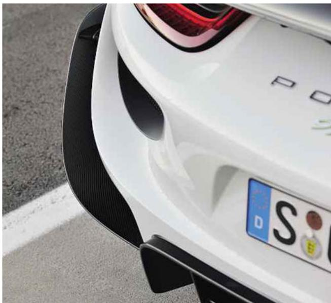
**Above:** rear aeroblades are among Weissach Package addenda. **Right:** V8's output goes to the rear axle only and is supported by an electric motor, so oversteer is always an option
