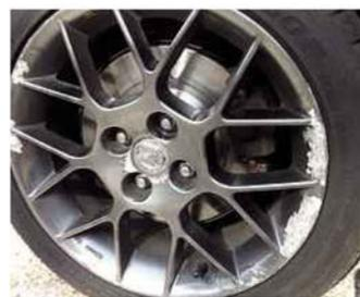
**Above:** MX-5's alloys were badly kerbed and corroded... **Below:** ...but a refurb has got them looking like new again
