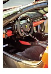
Left: seat position is fixed, so the almost-square wheel and the pedals adjust out to meet the driver. Bottom left: huge paddles operate dual-clutch transmission
