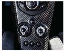
Above: P1's controls include twin dials for handling (H) and powertrain (P); both have Normal, Sport and Track settings. Above left: IPAS button gives an extra shot of power for those tricky overtakes
