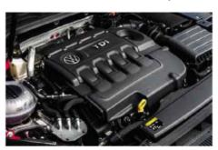
Above: 2-litre turbodiesel engines in both the 220d and Golf GTD produce identical outputs of 181bhp and 280lb ft
