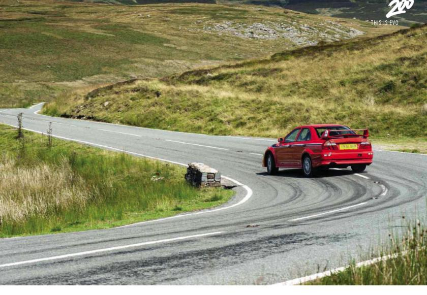
front end push, you sense that the Mäkinen is all done. But it isn't. Keep on the power and the four-wheel-drive system and the torquevectoring Active Yaw Control rear differential feeds the outside rear wheel with more torque, the understeer magically evaporates and the car adopts some angle at the rear.
