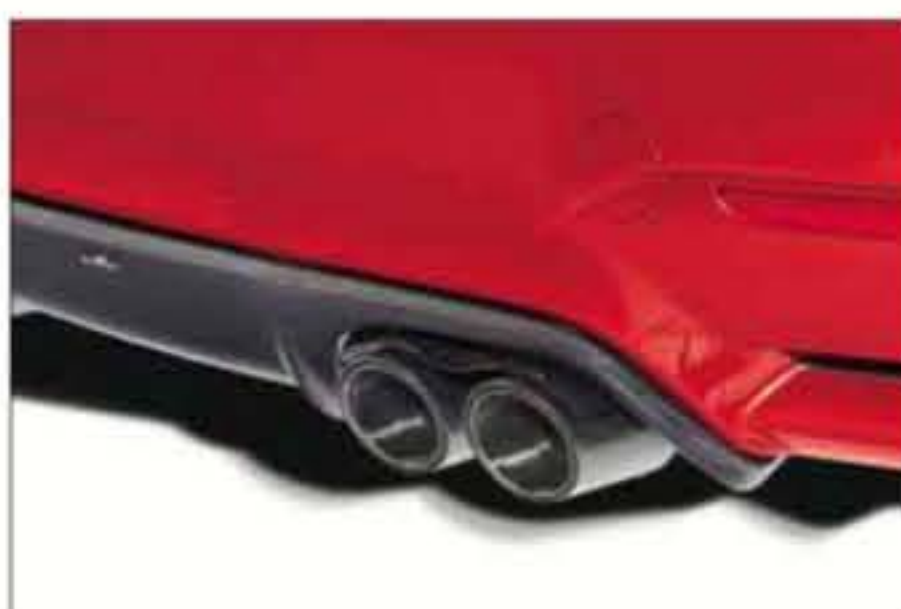
Quad sports exhaust with 90mm carbon fibre tailpipes & diffuser
