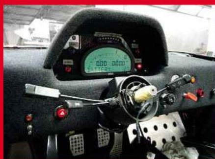
Above: modern Motec display replaces the road car's analogue dials in the binnacle. Right: five-speed 'box was rebuilt; the cogs for first and second gears were replaced to avoid potential problems from the stresses of racing
