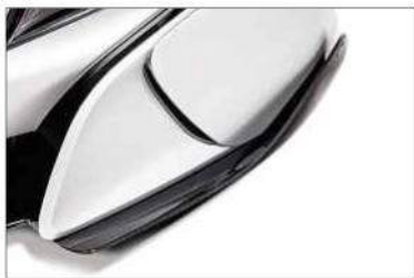
Carbon fibre front spoiler elements enhance aerodynamics
