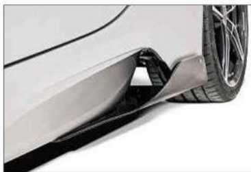
Carbon fibre side skirts divert air flow around the rear wheels
