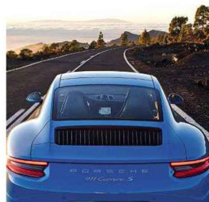
Right: slats on the rear are now vertically arranged to improve airflow. Below: smaller steering wheel is inspired by the 918 Spyder's; driving modes are selectable via a dial beneath the spokes
