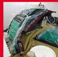
Below: carbon-Kevlar wheelarch linings were remade from scratch
