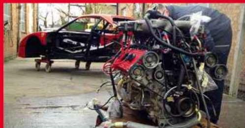
Left: with scored cylinder walls and big-end bearings, the engine needed a full rebuild.
