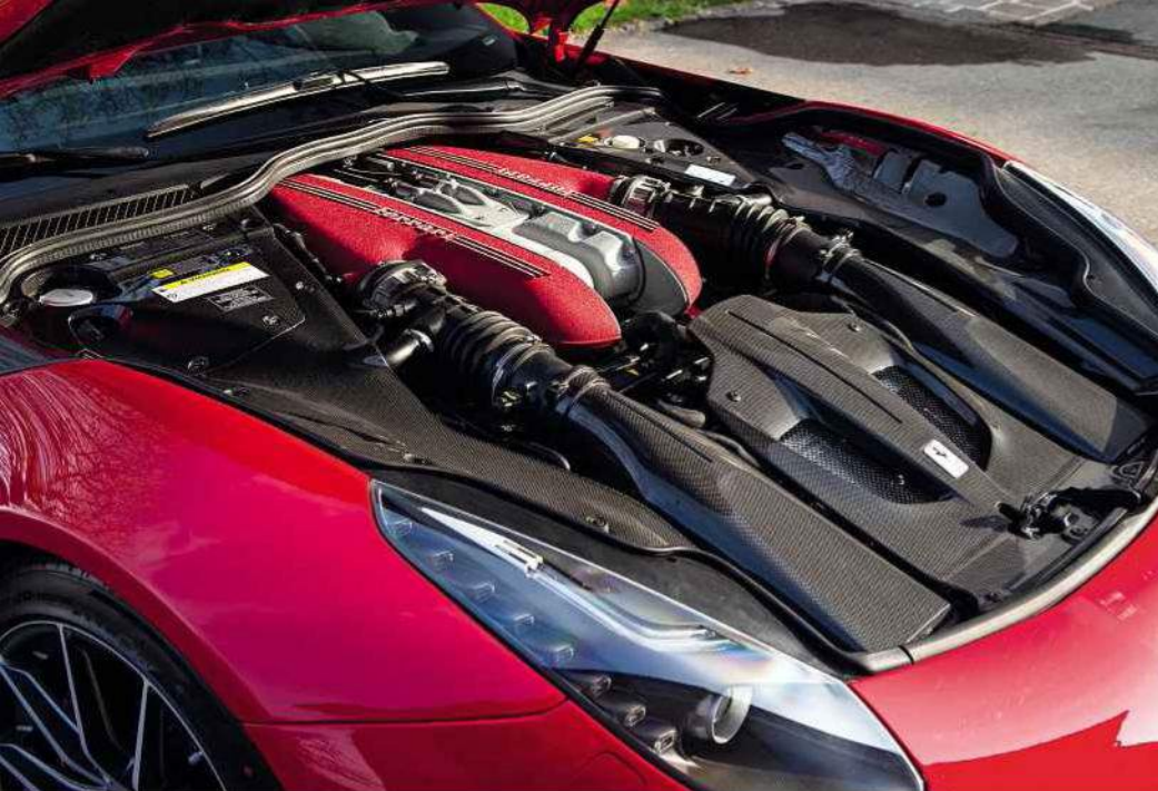
Left: changes to V12 include variable geometry intake system and race-style mechanical tappets. Below: rear wing vents help aero, look gorgeous
