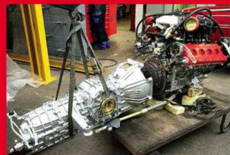
Above: modern Motec display replaces the road car's analogue dials in the binnacle. Right: five-speed 'box was rebuilt; the cogs for first and second gears were replaced to avoid potential problems from the stresses of racing
