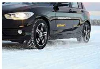
two per cent per millimetre from 8 to 4mm, but double that from 4 to 2mm. From 50kph (31mph) a tyre at the UK legal limit will need 26 metres longer to stop than a new one. Easily the difference between having a crash or avoiding one.
