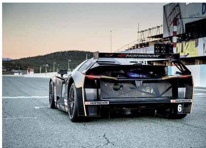
its most aggressive ride height, the X-Bow GT4 generates significant downforce, but the Balance of Performance ruling also stipulated a higher ride height to further limit its performance. The car is running in this setting when I sample it at Automotodrom Grobnik in Croatia.
