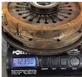
**Left:** the SC is in for a treat with WEVO's Streetlite clutch and flywheel, which uses AP Racing hardware and weighs roughly half what the OEM items do
