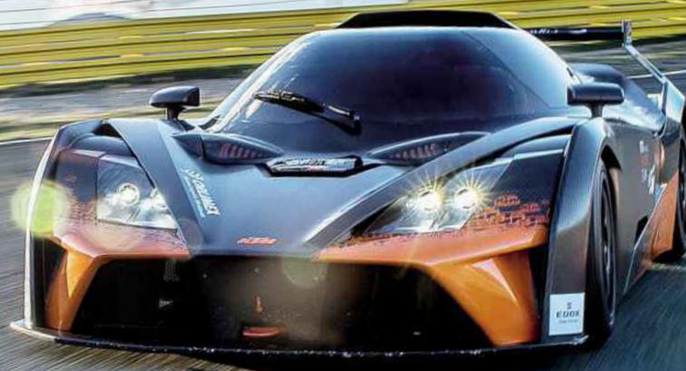
**T**HE KTM X-BOW HAS been used in competition ever since it entered production in 2008, but in the new X-Bow GT4 the Austrian manufacturer now has a purpose-built racing machine. It shares the road car's carbonfibre monocoque, 2-litre turbo engine and inboard suspension architecture, but with closed wheelarches and a full canopy it's lost that version's pared-back, exoskeleton styling.
