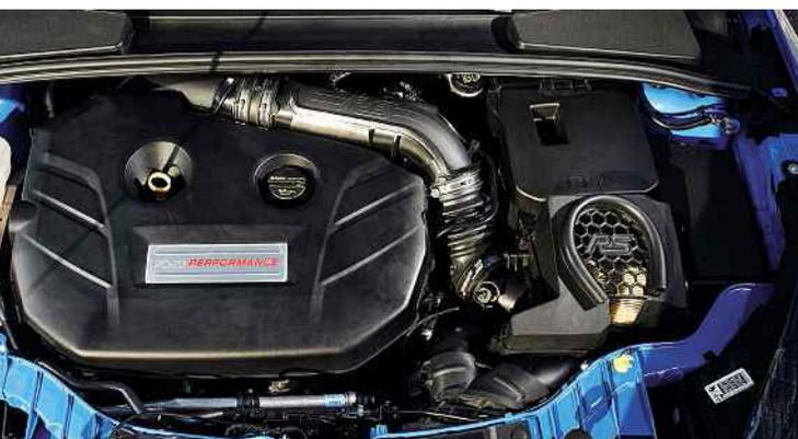
**Top:** 20-spoke wheels are optional; basic design has ten spokes but is the same 8 x 19in size. **Top right:** standard Recaros, complete with showy blue detailing. **Above:** 2.3-litre four has a twin-scroll turbo and puts out 345bhp; open air filter helps to maximise air-flow on rolling roads
