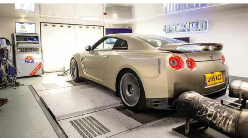
Above: dyno test put to bed any notion that our press-spec GT-R was somehow 'different' to normal ones; its 559bhp was a little more than the official 542bhp, but this isn't unusual
