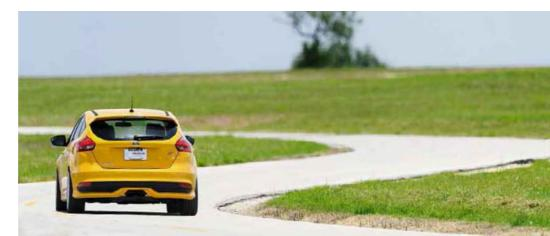
The Vredestein came second both in my subjective assessments and in terms of lap time. It recorded an average of 91.25sec, dropping just two-tenths to the Michelin. I rated the Vredestein highly for traction and stability in high-speed transient corners.
