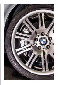
the rear, which is plenty for the M3. Also included are low-noise pads designed to operate when cold and eliminate squeal. I've driven the M3 through London and they haven't made a peep, which is impressive given the size of the discs (365mm at the front, up from 325mm).
