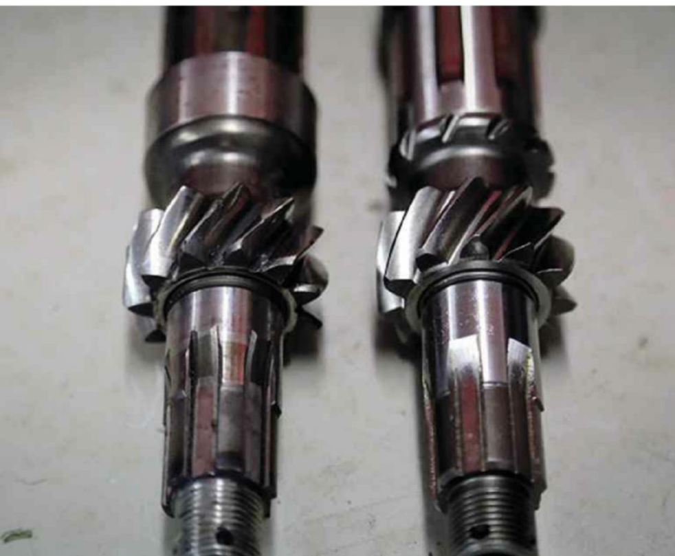
Left: the well-worn original first-gear input shaft (left) beside its replacement. Below: new crown wheel and pinion set will bring a lower final drive. Bottom: one of the graphs that helped Trott decide which ratio to plump for
