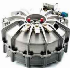
Left and above: Hill and Villeneuve dominated in the FW18 in '96. Below: Williams flywheel from the hybrid 911 GT3 R race car
