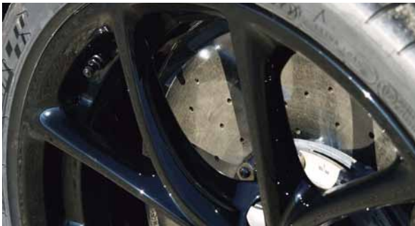
Above left: huge rear aerofoil changes angle depending on whether it's required to increase downforce for cornering, reduce drag for V-max runs, or act as an air brake to supplement the gargantuan carbon-ceramic discs (left)
