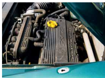
Above left: pared-down components and bare aluminium floor. Above: five-speed gearbox not quite as slick as Barker recalled. Left: 118bhp K-series engine still feels perfectly matched to flyweight Elise
