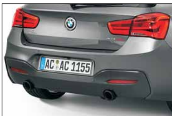
Hi-flow sports exhaust with 90mm tailpipes and valve control
