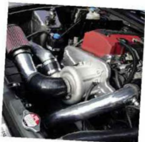
TTS Supercharged Honda S2000 Stock Performance 240Bhp/208ft-lb Torque
