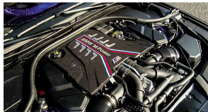
Above: 4.4-litre biturbo V8 from previous F10-gen M5 now makes extra 40bhp, lifting total to 592bhp; AWD traction means 0-62mph takes a mere 3.4sec
