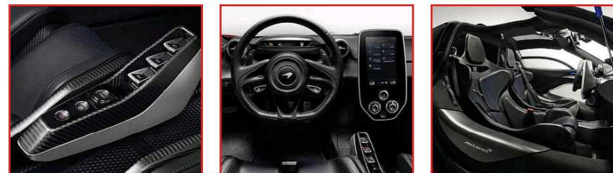
Above, from left: gear selector panel moves with seat; interior has been kept as simple as possible to minimise weight – hence lots of exposed carbonfibre; bucket seats can be specified with leather or Alcantara trim
