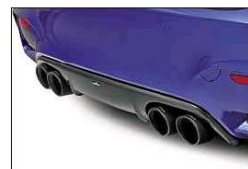
Hi-flow sports exhaust with 90mm tailpipes & carbon rear diffuser
