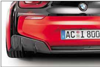
Three piece carbon rear diffuser helps move air from underneath
