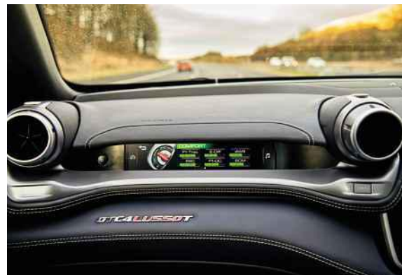
Above: optional 'co-driver' touchscreen can display current drive settings or performance data, or control the infotainment system
