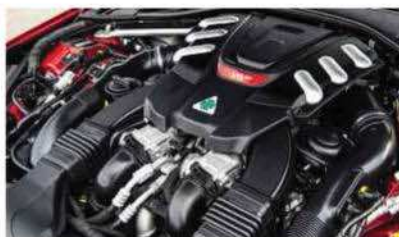
Above: twin-turbo V6 puts out 585bhp thanks to ECU tweaks; a 660bhp upgrade is in the works
