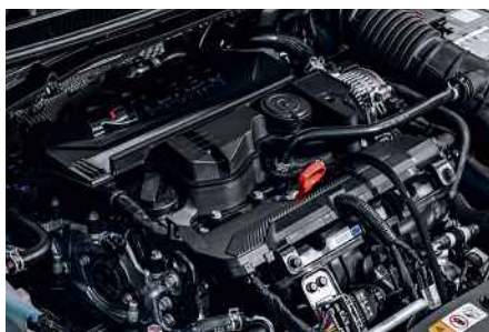
Above: 201bhp and 203lb ft 1.6-litre four is a pepped-up version of the unit found in Kia's Ceed GT and Proceed GT. Right: steering wheel home to 'N' mode switches and a red button to engage rev-matching
