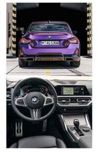
Top: 19-inch wheels are standard, as are uprated M Sport brakes. Above: interior is suitably driver-orientated, but no manual gearlever or third pedal - the M240i is auto only
