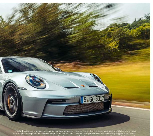
a Carrera, but the operating window in terms of height and the angles it reaches is bespoke to the Touring to make sure it develops the same level of stability as the GT3's distinctive swan-neck item. With modifications to the front splitter, underfloor aero and the rear diffuser, Porsche's claim is that stability and aero performance is as near as dammit identical whether you go for a wing or a spoiler.
