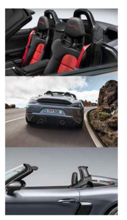
Above: ultra-lightweight soft-top arrangement includes a 'bimini' top for sun protection; carbon-shelled sports seats feature Race-Tex centres; in place of the GT4 RS coupe's high-mounted rear wing, the Spyder RS has a slightly more subtle integrated ducktail spoiler
