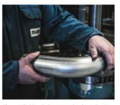
**Above:** Milltek has the largest pipe benders in the UK exhaust industry, capable of working 102mm diameter tube. **Top:** complete system for a 911. **Left:** systems are currently in development for new Civic Type R and Emira
