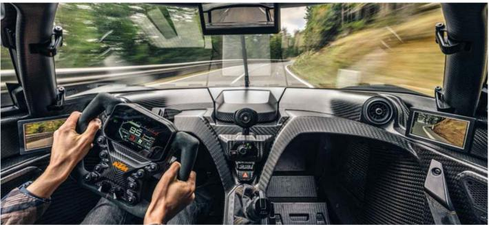
Clockwise from top left: cockpit is accessed via electrically powered canopy; once open it also reveals pushrod-operated inboard dampers; no rear-view mirrors so driver has three camera screens instead
