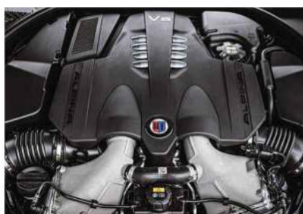
Above: twin-turbocharged 4.4-litre V8 produces 89bhp and 37lb ft more than in BMW's M850i, taking the total outputs to an M8-rivalling 612bhp and 590lb ft
