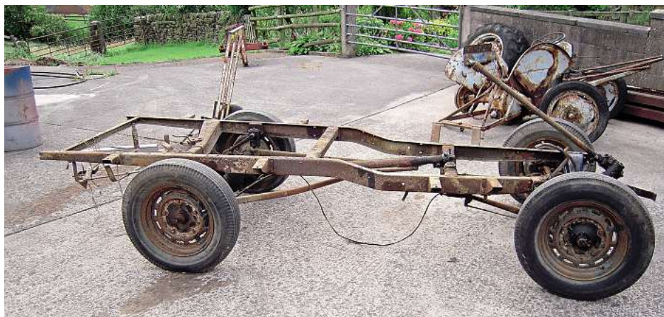
All stripped down to a chassis and wheels showing the original construction that's in great condition.
