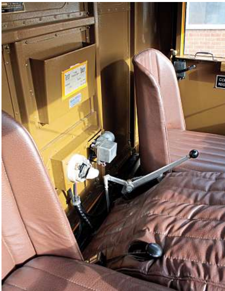
The extra lever is to operate the pump discharge via the engine driven pto.
