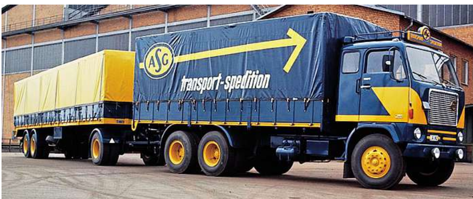
Ideal for the longer-length combinations allowed in Sweden, the set-forward axle G Series was also available in three-axle G89 spec.
