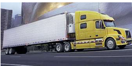
This long-hood, 77in sleeper cab VNL 780, available with 355-600bhp engine options, is Volvo USA's flagship.
