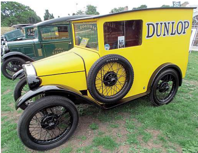
Jeffrey Blight's 1929 Dunlop replica van has a completely coachbuilt body. Note the lack of a passenger door.
