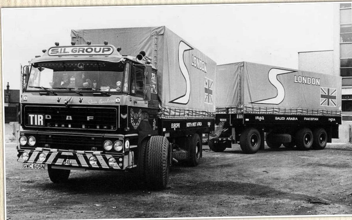
LEFT: This is apparently the 'Desert DAF'. The caption on the back of this press photo says it's the first FA2800DKS 'road train', and the front axle is fitted with super-singles when in the desert.
