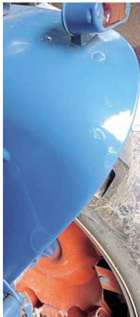
16 This tractor wing was painted about seven years ago, after discovering rust fingers spreading under the panel holding coat as supplied on replacement wings, it was rubbed down to bare metal and treated with zinc phosphate. There are no signs of any rust activity under the paint.
