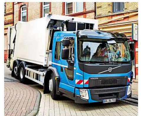
Another current spec, the FE, features a walk-through cab and a kneeling function that lowers step height from 800mm to 440mm.
