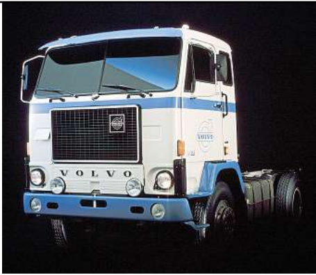
With evident US cabover influences, the two-axle F88 became the prototype for all successive European heavies.
