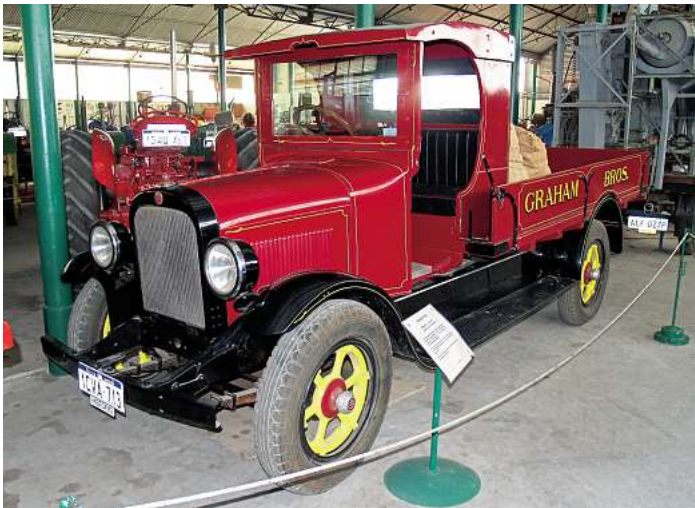
The Graham Brothers started converting Ford Model Ts into trucks in 1908. This type was built between 1921 and 1925 and is fitted with a four-cylinder Dodge engine.
