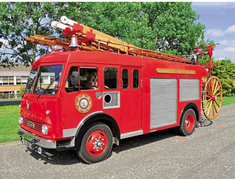
ASK 701C has the early TK model split screen, which bearing in mind the 1965 registration seems a bit of an anomaly. But according to Jim it was common practice for fire engines to be acquired and stored for several years, before finally being registered.
