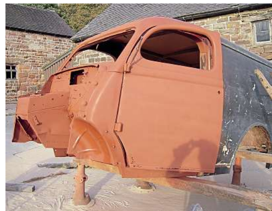
All sandblasted on site, the cab has primer applied before repairs are made to the nearside door, which features a number of former rusted areas.
