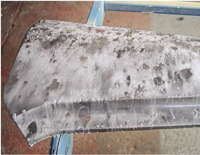
10 Sometimes areas will bubble up during the process, this is perfectly normal, just keep the surface wet, the blurb says if used on surface rust leave for 30 min, but leave for a minimum of 20 minutes on clean panels.
