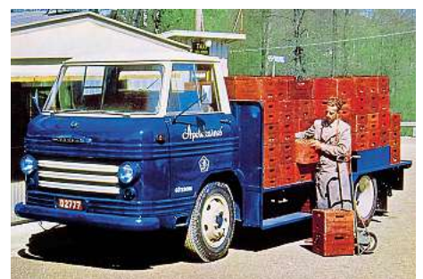
The L430 Trygge five-tonner was introduced in 1957, initially with a petrol engine, and a 65bhp Ford diesel from 1963.
