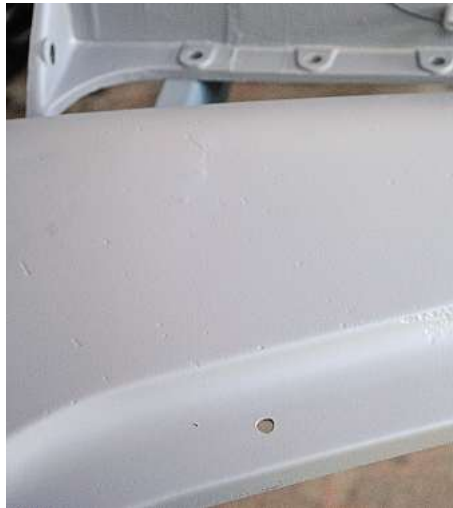
13 Once the steel panel had a coat of primer, it clearly showed the pits where the rust had been, these small blemishes are easily remedied, with the application of some acrylic putty before further coats of paint.
