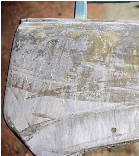
12 Once dry, the zinc phosphate can clearly be seen on the panel surface, this will keep rust at bay, but it will be best to get some more paint on fairly quickly.
