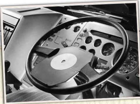
Did you know that the steering wheel centre on the Leyland DAF 95 folds out into a 'document table'?
