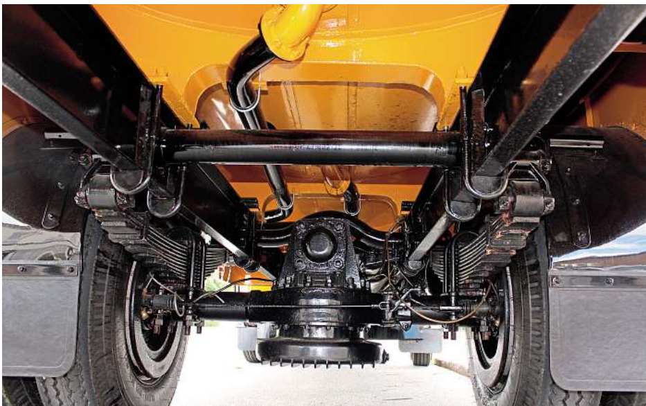
Even the underneath is great – and we love the shape of the heavy-duty Albion diff casing.
