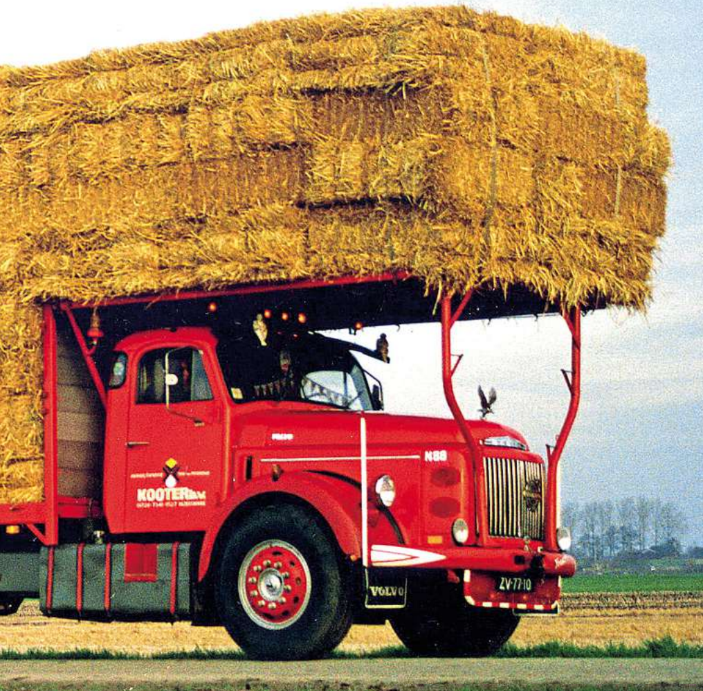
Heavy-duty N88 Series trucks had seven- or 10-litre turbodiesels and were technically sophisticated in every respect.
