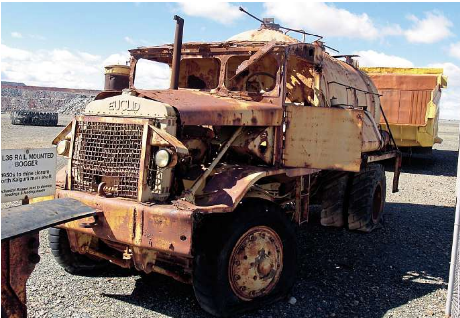
This Euclid had been converted from a dumper into a water tanker for an opencast gold mine.
