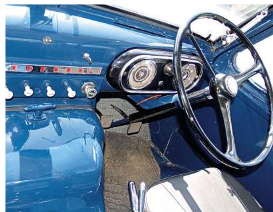
It's just as immaculate inside. Note the knob on the right of the centre panel for the Ki-Gass.
