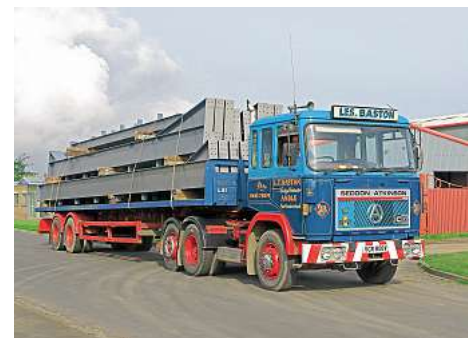
A common upgrade was to fit the later 401 grille on to your old 400, as done here by Les Baston, together with many other modifications. PHOTO ALAN BARNES.
