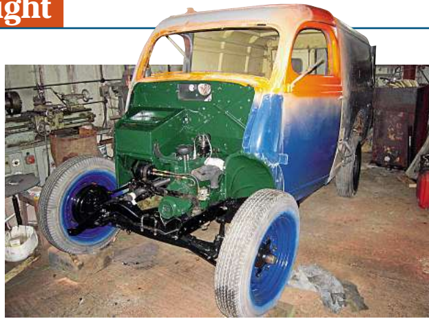
The reconditioned 10hp engine in place and the body can be lowered on.
