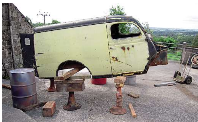
All up in the air with the bodywork removed by jacking it off the mountings.
