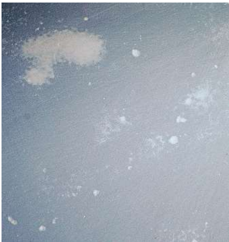
15 Once the fine filler is dry, rub down with fine abrasive (400 grit wet and dry) all those pits can be seen as a lighter shade, now filled, a few needed a second going over before applying more undercoats.
