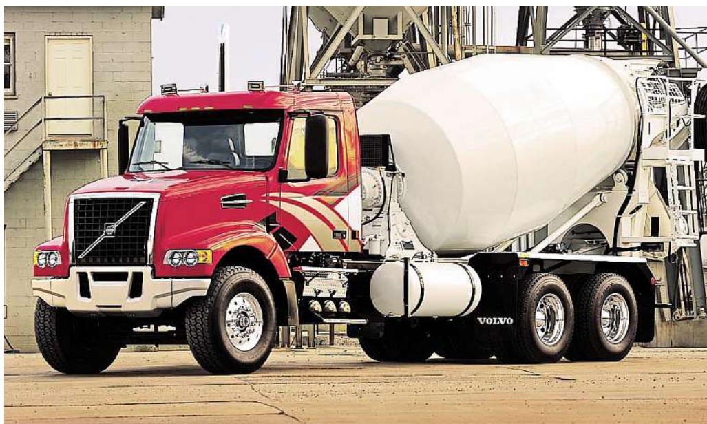
The Volvo VHD is aimed at North American vocational rigid truck markets. Engine choices offer up to 500bhp/1850lb-ft maximum outputs.
