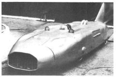
Land Speed Record monster—Eyston's famous "Thunderbolt", all 73-litres and nearly seven tons of it, in its 1937 form, with open cockpit and cowled radiator. It ran on eight Dunlop-shod wheels and broke the LSR on three occusions, saking it to 3574 m.ph. by 1938.
