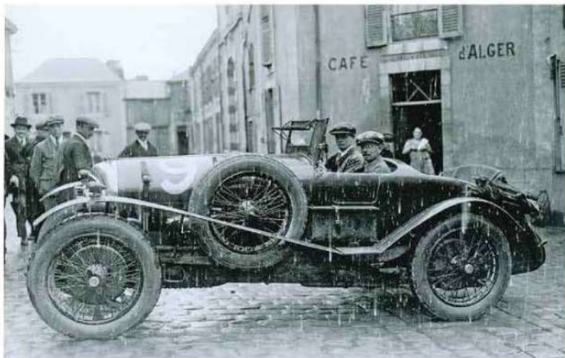
Above and right Period shot shows number 9 after scrutineering for the 1926 Le Mans 24 Hours; no driver's door because the gearlever is in the way.
