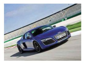
TOP OF AUDI'S revised R8 model range is the faster, lighter, sharper-handling R8 V10 Plus. Available only as a Coupé, the £127,575 Plus weighs 50kg less than the regular V10 thanks to standard carbon ceramic brakes and more carbonfibre components in the body. Power and torque have been boosted by 24bhp and 7lb ft, lifting maximum output of its howling 5.2-litre V10 engine to 542bhp and 398lb ft.
