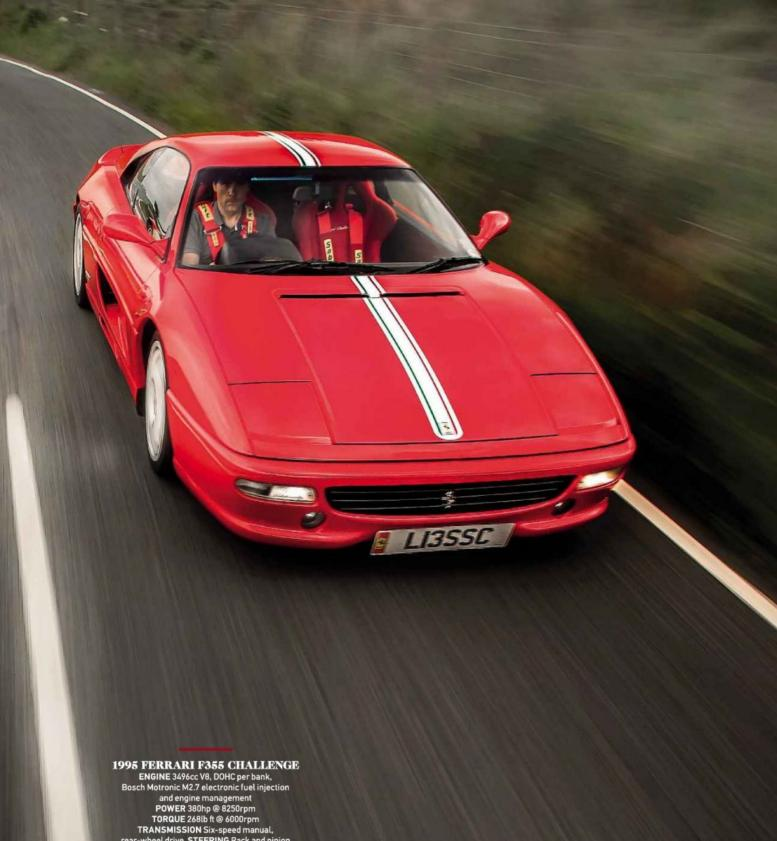
Bosch Motronic M2.7 electronic fuel injection and engine management POWER 380hp @ 8250rpm TORQUE 268lb ft @ 6000rpm TRANSMISSION Six-speed manual, rear-wheel drive STEERING Rack and pinion SUSPENSION Front and rear: Unequal-length double wishbones, coil springs, telescopic dampers, anti-roll bar BRAKES Ventilated discs WEIGHT 1335kg PEREORMANCE Top speed c183mph. PERFORMANCE Top speed c183mph. 0-60mph c4.3sec
