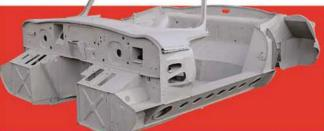
SUB ASSEMBLY UNITS SERIES I, II AND III A body shell without the outer panels fitted, complete with new bulkhead fitted:
