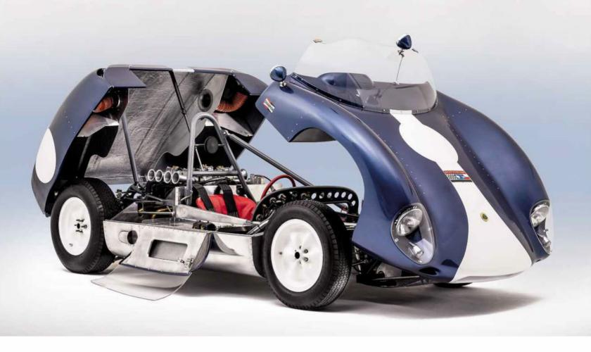
With an eye to modern safety, Tolman installed rollover protection with a T45 roll hoop combining fore and aft location stressed correctly. In addition, the floor was not simply an alloy skin but a high-strength aircraft alloy, riveted and bonded along the bottom for greater safety. The fuel system again was custom designed, incorporating a one-off Tolman-designed ATL fuel cell; even the pipework has a classic influence, being all black and cloth-wrapped where appropriate.
