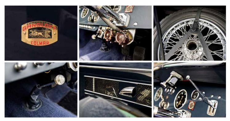
being a late-series 57, its engine is rubber-mounted for smoothness. Furthermore, the Bugatti benefits from hydraulically operated drum brakes and a stiffer chassis. But as part of cost-cutting exercises, the 57 does without the previous, expensive Bugatti alloy wheels with integrated drums and instead features centre-mounted Rudge Whitworth wire wheels.
