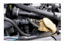
wash leather, secured with a cable tie (thank goodness Harry had left a packet of them in the boot), it would leave the system unpressurised and able to breathe, while still preventing water from splashing out. And I could reinforce my duct-tape hose repair with a couple of dozen more cable ties.
