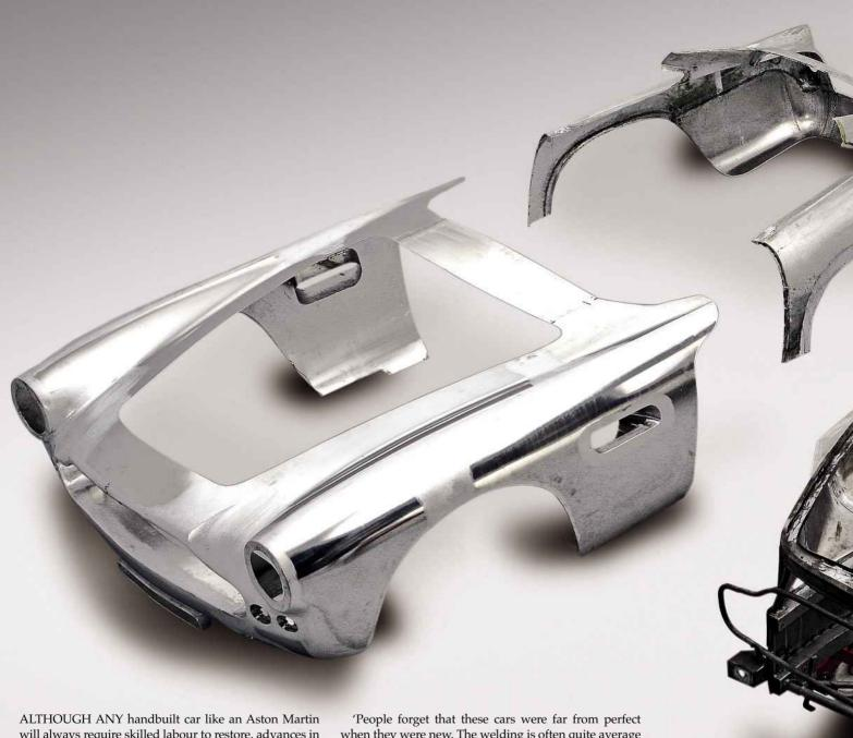
will always require skilled labour to restore, advances in technology have made it easier to achieve really durable and consistent results. For example, at Aston Engineering, after the chassis and Superleggera framework have been shotblasted, instead of being painted in red-oxide as they were at the factory, the bare metal is now powdercoated with a semi-matt black and very tough chip-resistant coating, which is electrostatically attracted into every nook and cranny.
