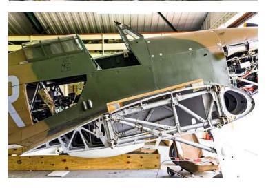
together with minimal riveting and no welding, the aeroplane could be assembled almost anywhere using relatively unskilled labour and without elaborate jigs to ensure accuracy. The clever bit was the design and the machining of parts.
