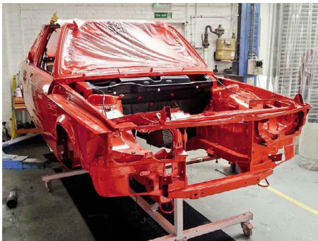
Clockwise from above Refinished underside gains new heat shielding; bodyshell looks like new in shiny red, with all rust surgically removed; engine needed just a check and a clean.
