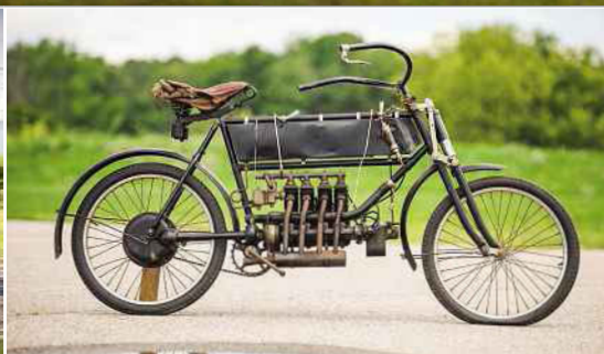
1907 Fabrique-Nationale Four 362-cc shaft-drive four-cylinder engine Frame No. 18074
