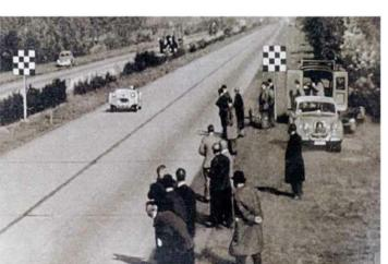
Facing page and below 'Guillotine-like' tonneau cover, aeroscreens and rear-wheel spats streamlined MVC 575 to the degree that it achieved nearly 125mph at Jabbeke in 1953.
