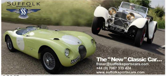
Suffolk C-Type Jaguar On the left, our new and improved Suffolk C-Type Jaguar with a fast road 4.2XK engine, our C-Type space frame chassis, disc brakes, torsion bar front suspension and Jaguar live axle. This vehicle is presented in primrose yellow with teal blue seats. We can build you a new car to your specification and in any colour you like.
