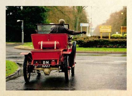
produces some alarming noises. If you're feeling especially confident, you can partially engage the ratchet on the outside lever to apply consistent braking force ahead of a junction, which frees up your right hand to make a downchange.
