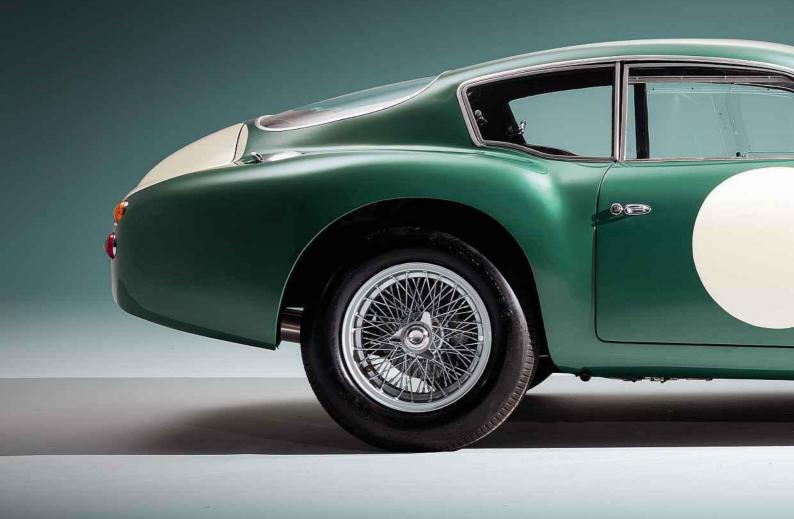
years, 2 VEV is back on the correct 16in Borranis, which are shod with Dunlop L-section racing tyres.
