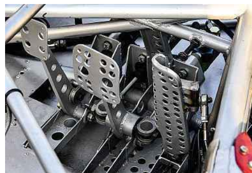
Left and below Right-hand gearshift features wooden knob and exposed linkage; adjustable drilled pedals feature in ultra-sparse cockpit.
