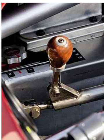
Left and below Right-hand gearshift features wooden knob and exposed linkage; adjustable drilled pedals feature in ultra-sparse cockpit.
