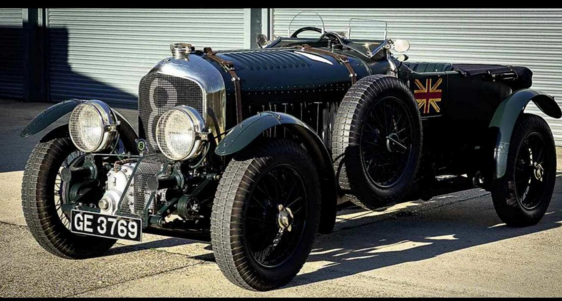
1929 Bentley 4.5 Litre Chassis UK 3299. A superb rebuild to full "Birkin Blower" specification. Le Mans Coachwork. Phoenix Crankshaft Rods and Rockers. Le Mans Fuel Tank & Instruments.
