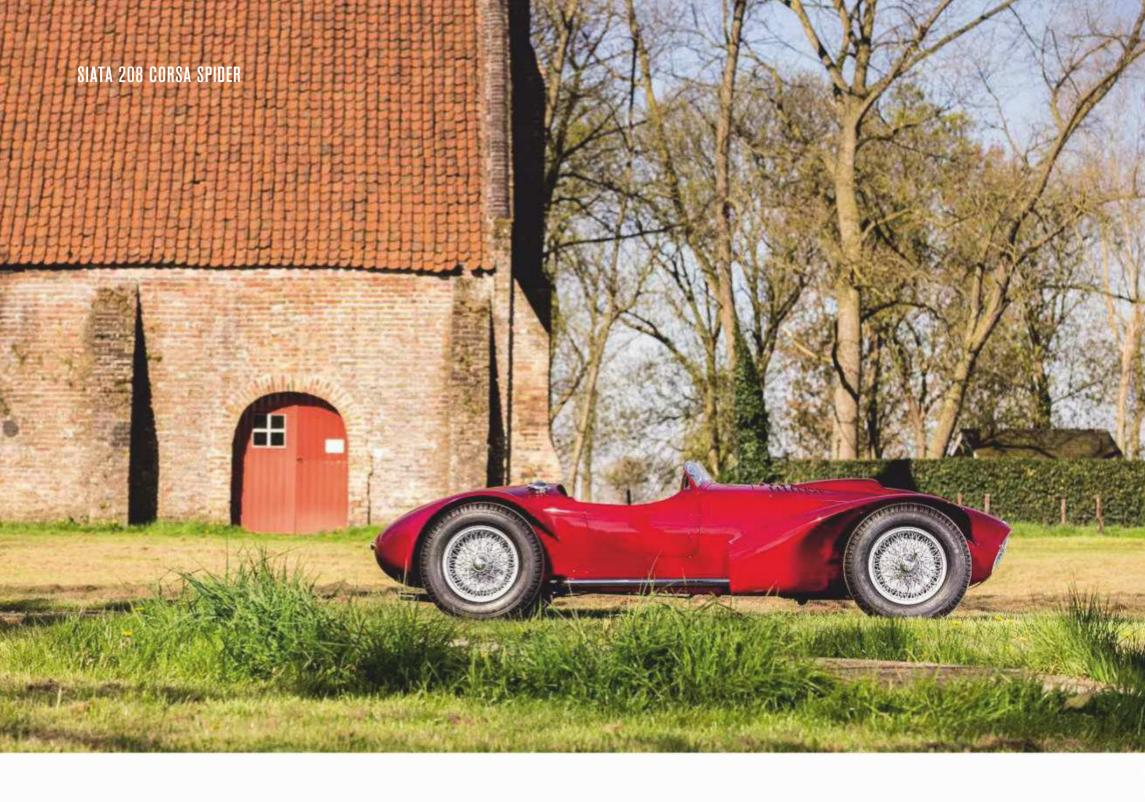
1952 Siata 208 Spider Corsa Engine 1996cc 70° V8, OHV, aluminium block and heads, two Weber 36 DC3 carburettors Power 160bhp @ 6000rpm Torque 130lb ft @ 4500rpm (est) Transmission Five-speed manual gearbox, rear-wheel drive Steering Worm and roller Suspension Front and rear: enclosed coil-spring and lever-arm damper units forming upper links, lower wishbones, anti-roll bar at front Brakes Drums Weight 680kg (est) Top speed 120mph (est) 0-60mph 8sec (est)
