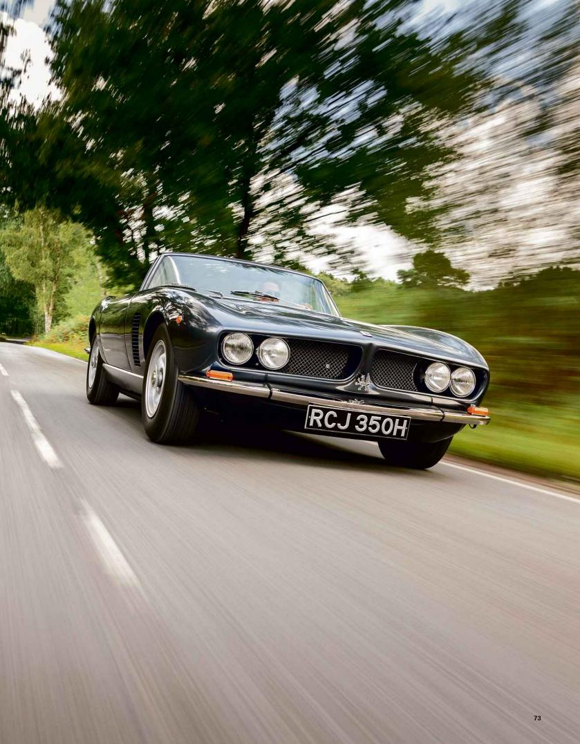
bluster was extinguished by the 1970s oil crisis. During that time the Grifo had three different gearboxes (four-speed Borg Warner, or fivespeed manual or three-speed auto from ZF), four engine variations (327, 427 or 454 Chevy or Ford 351) ranging from 5.4 to 7.4 litres capacity, and
