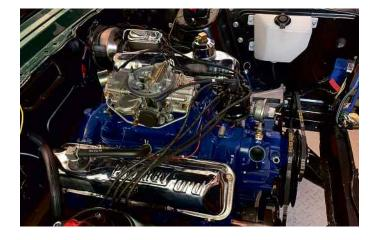
Once the engine was stripped, I took it to Chesman Engineering in Coventry for machining. The crank was in good condition and need only a 10 thou' grind but the bores, while standard size, were extremely worn, no doubt due to playtime on the ranch with no air filter. The camshaft was an easy fix, thanks to Crane, which lists the original, and I found a pair of genuine, cast iron, 14-stud GT exhaust manifolds on eBay.
