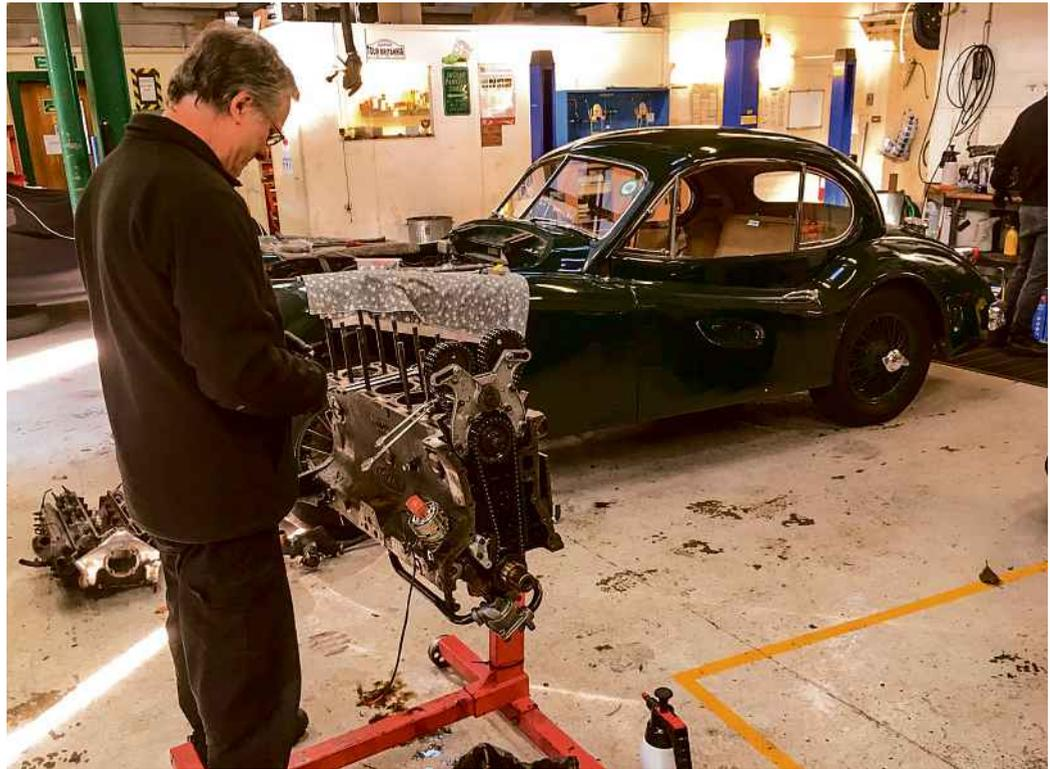
I'D TAKEN THE Jaguar down to Twyford Moors for a clutch upgrade – pretty standard stuff, except that with an XK140 it's an engine-out job. And an XK lump requires quite a degree of heavy lifting. So, with the engine removed, I casually asked Ian and the team to take a look at the lazy chain tensioner, as it's apparently easier to get at the front engine cover with the engine on a stand.
