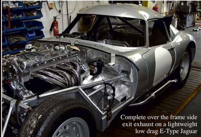
Complete over the frame side exit exhaust on a lightweight low drag E-Type Jaguar
