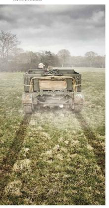
Narrow tracks are required to allow 'warp steering' but, even so, the Carrier's light weight means it's less likely to sink into waterlogged ground, as here.
