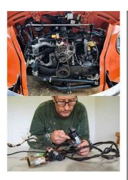
enthusiasm to finish the Beetle was revived and when we looked at the list of jobs left to do it came down to this: finish fitting the replacement VW loom, fit the cut-down Subaru loom we'd had made, fill the cooling system and plumb in the injection fuel pump.
