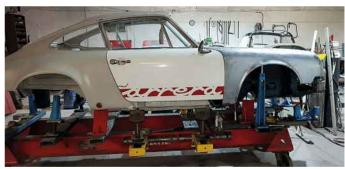
pressing for what was intended to be a limited-volume run, Porsche achieved the extra wing width by taking a standard 911 panel, cutting out a substantial arc of metal and welding in the new flared shape. This left a telltale seam on the inner surface and it is not unknown for RSs to have been restored with the incorrect profile on the rear wings.
